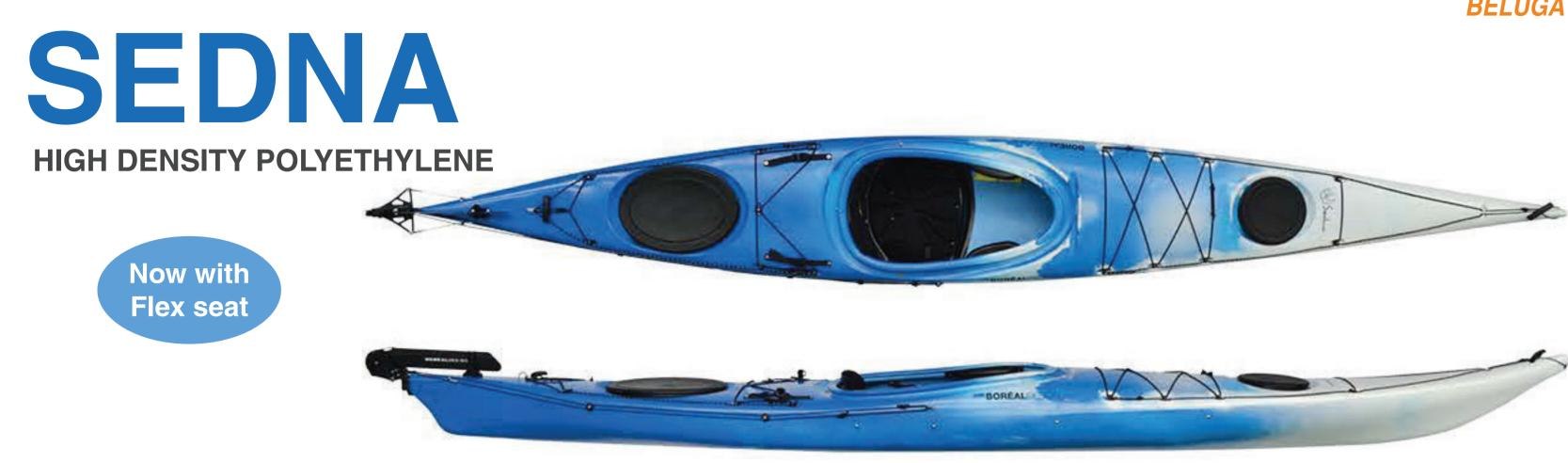
The Sedna is one of our most versatile models. Its arched hull shape and waterline length have been designed to provide stability combined with very predictable behavior, as well as easy handling while requiring a minimum effort to maintain a good cruising speed. These characteristics are sure to appeal to the day or weekend paddler who loves to go exploring in all types of weather and water conditions without the storing inconvenience of a 17ft kayak. Comes standard with a rudder system.
