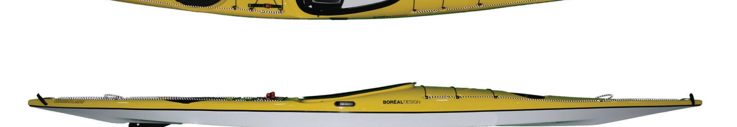
The Norsaq is the first of its kind: a pure Norsaq made from our highly durable, sleek finish and affordable thermoformed ABS material. Inspired by traditional designs and influenced by the possibilities of our thermoforming construction, this kayak was designed to be the perfect boat for a mid to large-sized paddler wanting
